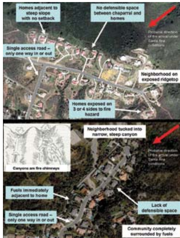
Figure 2. Many California housing tracts violate basic principles of fire safety in high-fire hazard areas. Topography is a major factor influencing home safety. Homes built atop topographic high points require setbacks from steep slopes, as wind-driven flames and convective heat can impact these homes directly.
